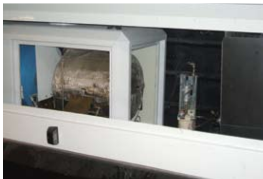
Capstone microturbines generate electricity to charge batteries on HEV buses, even running on jet fuel if needed.
